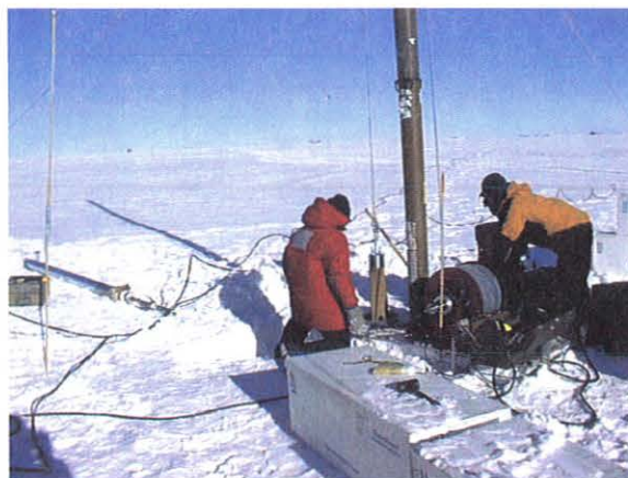
Fig. 5.42. Bladder being sent down into one of the two holes at South Pole for subsequent sampling of firn air. The 10-m-long bladder was pressurized to inhibit airflow from above while firn air was sampled through a 15-cm-high, stainless-steel-lined open chamber situated between the bottom of the bladder and the bottom of the hole. Each of two holes, extending ultimately to the snow-ice transition at 122-m depth, was drilled and sampled at 2- to 10-m increments. The drill lies on the snow to the left.
