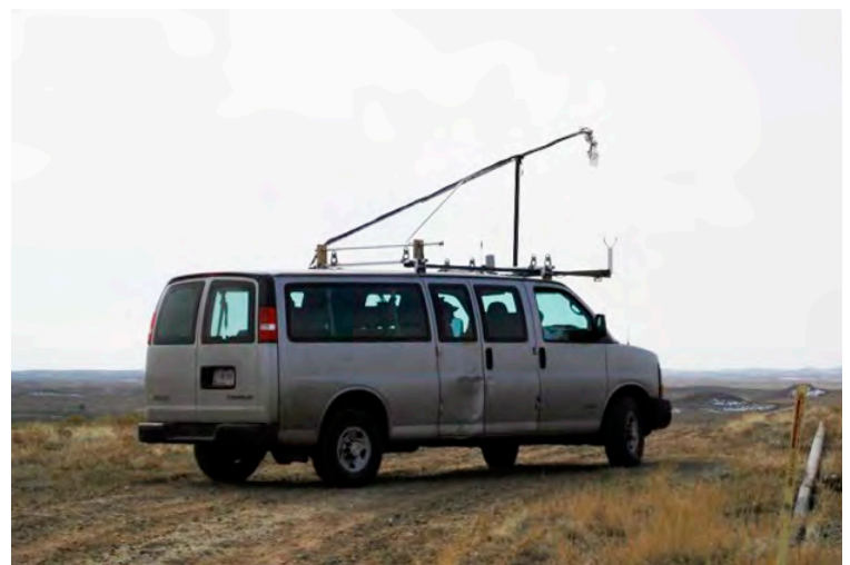
Photo above: Mobile sampling lab. Photo (Top Right): Gaby Petron tells U.S. Rep. Jared Polis how she uses the mobile lab to monitor conditions in local oil and gas fields i.e. in Utah (Bottom Right).
