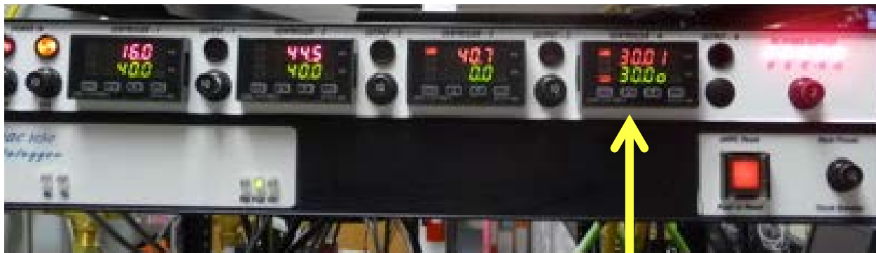
PID Flow Control
