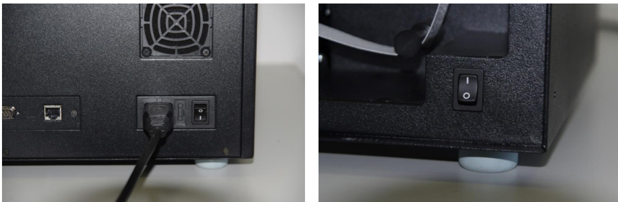
Figure 5. Power on switches: rear panel and inside the door on the right.
