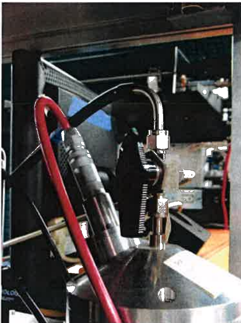
Figure 1 – zero/flowcheck valve (zero position)
