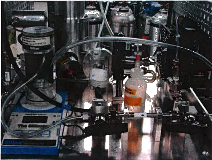
Figure 5 - sheath air valves in sheath air flowcheck position
