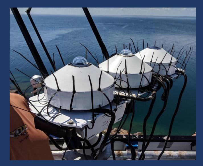
A temporary solution is using tie wraps to deter seagulls from perching on the domes.
