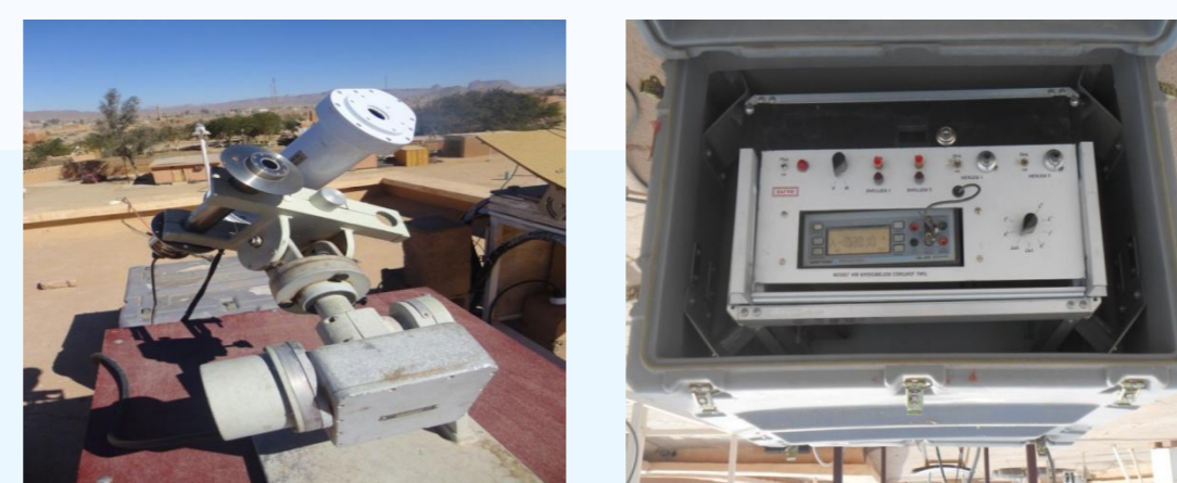
Fig.4. Pyrheliometer mounted on AHF Cavity & Radiometer Control Box.
