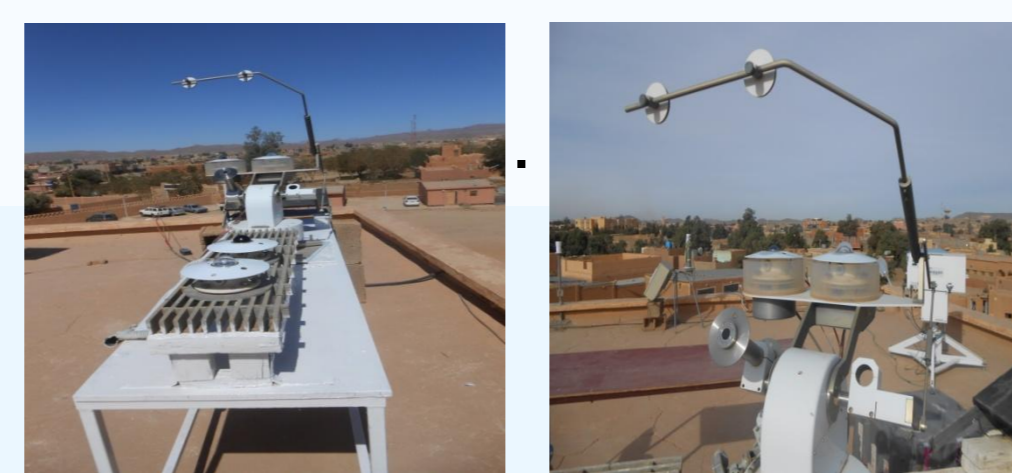
Fig.2. Solar & thermal radiation instruments installed on the roof.
