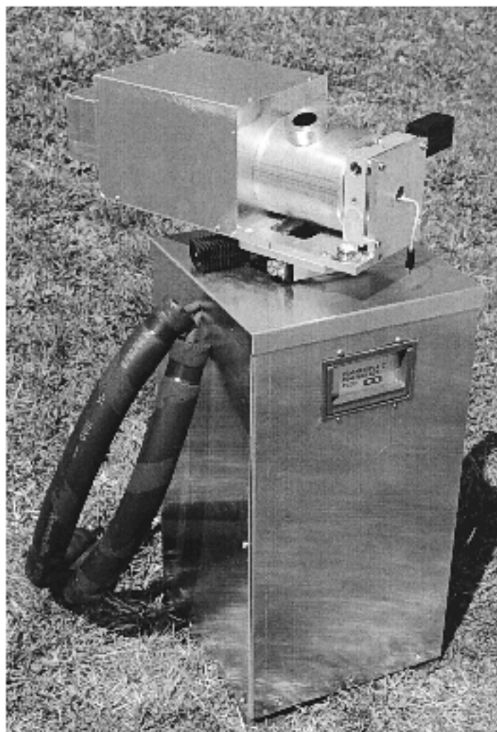
Fig. 2. ASR with reference blackbody (lower part) and rotatable detector head (upper part).
