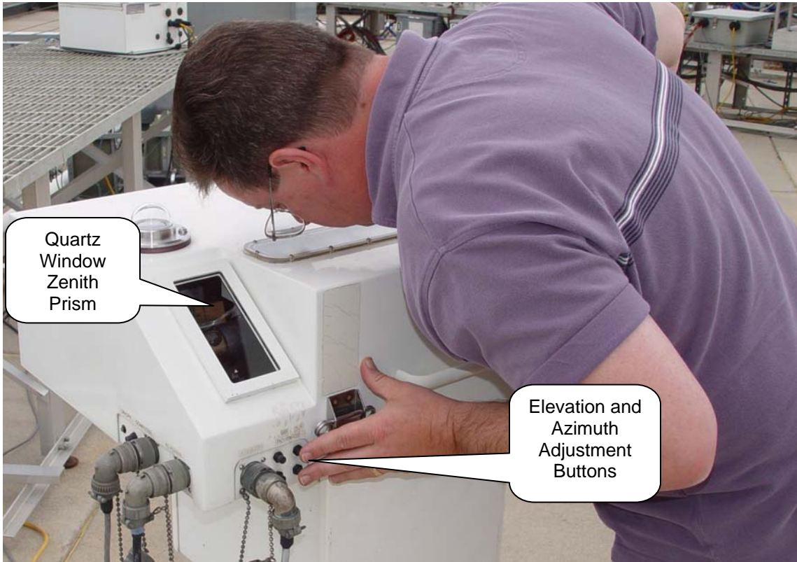
Figure 4-16 Looking through sighting tubes without blocking the Quartz Window from the Sun
