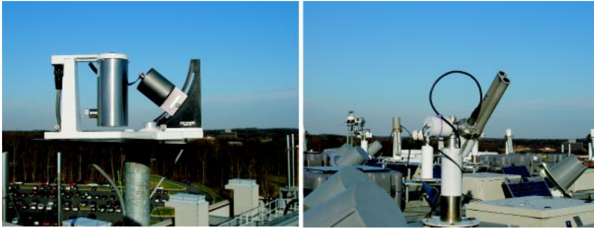
Fig. 1 UV-MFRSR shadowband radiometer, part of USDA UVMRP (left), and CIMEL sun/sky photometer, part of NASA AERONET network (right) were continuously run side by side at NASA GSFC in Greenbelt, Maryland (lat=39.03 deg N, long=76.88 deg W), in 2002 to 2004. The elevated location (the height of elevated platform at the roof of the building is \sim 20 m above ground and \sim 90 m above sea level) enables unobscured view of horizon by both instruments.
