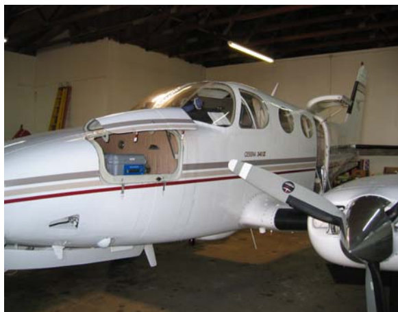
Figure 1. Trinidad Head aircraft in the Brookings, Oregon, hanger with 2B Technologies, Inc. ozone instrument shown in front luggage compartment.
