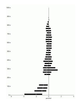
**Figure 1.** Frequency distribution (25-percentile/median/75-percentile) of the deviation between the mid-PBL  $CO_2$  mole fraction and the mole fraction measured at a given elevation above the ground in summer half year (April-September).
