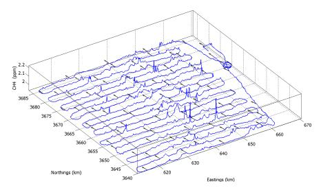
**Figure 1.** Raw methane concentration data from Flight 1007, showing correlation of local concentration anomalies with air movement vectors (black arrows). The flight area is 45x45km and aircraft flew at 165m altitude.
