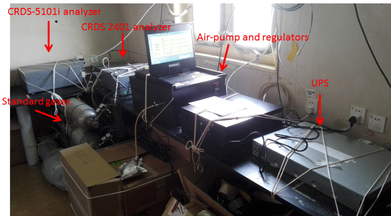
Measurement system in the atmospheric Lab N 2 O mixing ratio was measured every 4-10 s by a CRDS 5101i analyzer. CO 2 /CH 4 /CO mixing ratios was measured every 5 s by a CRDS 2401 analyzer.
