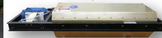
GSFC Compact Formaldehyde Fluorescence Experiment (COFFEE) measures atmospheric HCHO located in the center of the pod
