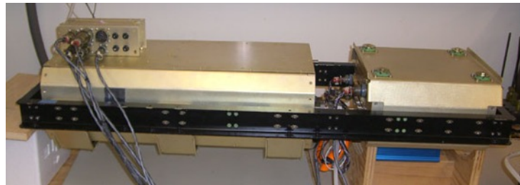
Modified Picarro (2301-m) measures \text{CO}_2 and \text{CH}_4 located in center- and tail-sections of the wing-pod
