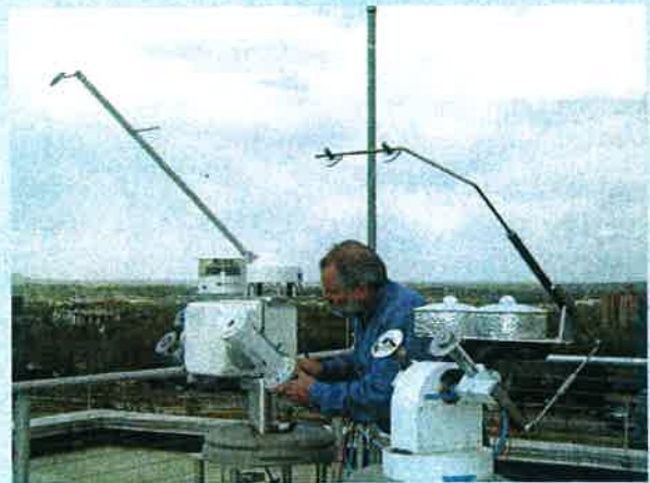
The operation of the CMDL primary solar calibration standard and associated radiometers is being checked in preparation for clear-sky conditions.
