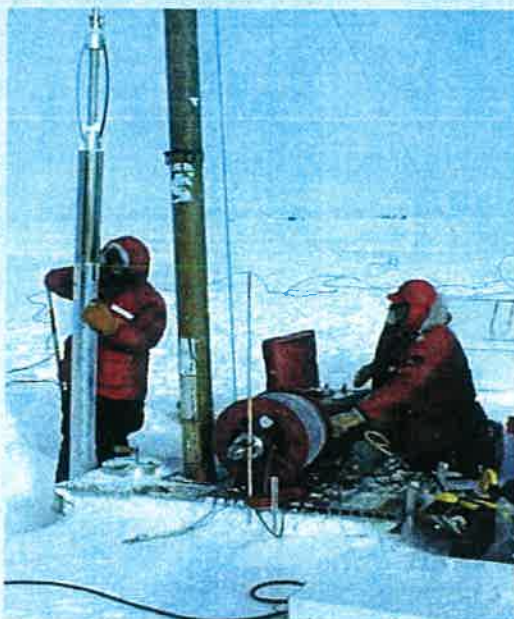
CMDL and collaborators sampling century old air from the South Pole snowpack.
