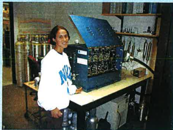
A 12-compound gas chromatograph developed and built by CMDL for operation at the baseline stations.
