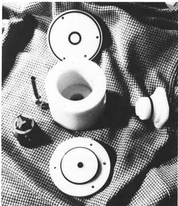
Figure 103.--Components of the Delrin housing for stage IV of the May (1945) impactor. This 10-cm-diameter housing seals the impactor to facilitate airborne use.
