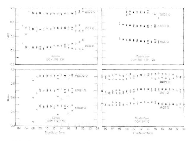
Figure 47. Ratios of solar irradiance measured through broad-band filters to total irradiance (quartz) for selected clear days. The difference between ratios is the contribution of solar irradiance between the spectral bands to the total solar irradiance measured, expressed as a percentage.
