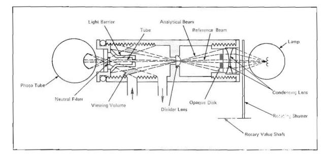
Figure 15. Expansion chamber and optics for the G.E. condensation nucleus counter.
