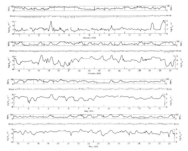
Figure 19. Hourly averages of 550 nm light scattering and relative humidity at MLO for January and May 1976. Wind speed and direction are given at 3-hour intervals. Speed is shown as the length of the vector where the barb length is equivalent to 5 kurts (2.6 m s<sup>-1</sup>).
