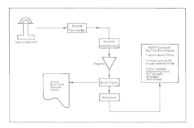
Figure 42. Schematic flow of measurement and recording systems for GMCC solar radiation instruments.
