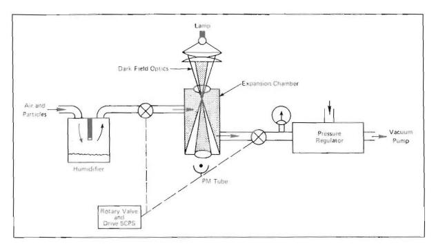
Figure 14. Diagram of air flow in the G.E. condensation nucleus counter.
