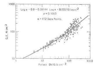
Figure 31. Comparison between Pollak counter SN15 and G.E. counter at South Pole for January to March and August to December 1976. Solid curve shows linear regression curve used to calibrate the G.E. counter.
