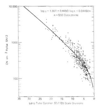
Figure 18. Comparison between longtube Gardner counter \$N1185 and Pollak counter SN13 on ambient aerosol at MLO during December 1975 and January to May 1976. The curve is a least squares fit of Hoerl's equation.
