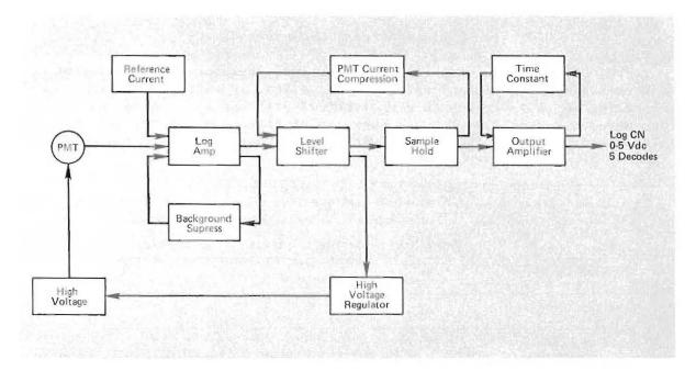
Figure 13. Electronic scheme of the modified G.E. condensation nucleus counter.
