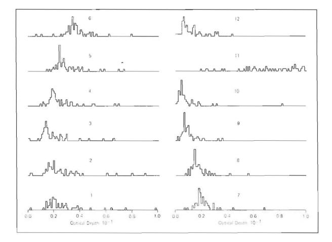
Figure A.2. Frequency distribution for ozone-plus-aerosol optical thickness at MLO for 85 days from March to August 1977. The numbers are sampled wavelengths numbered sequentially from blue to red: No. 1, 401 nm; No. 2, 422 nm; No. 3, 486 nm; No. 4, 521 nm; No. 5, 537 nm; No. 6, 611 nm; No. 7, 659 nm; No. 8, 669 nm; No. 9, 750 nm; No. 10, 860 nm; No. 11, 947 nm; No. 12, 1010 nm.
